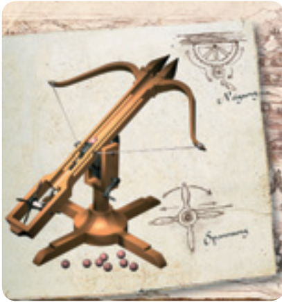
This crossbow designed by the Renaissance genius Leonardo da Vinci (1452-1519) worked on the same principle as our shot put machine. Deciding factors when making a shot are angle and tension.
