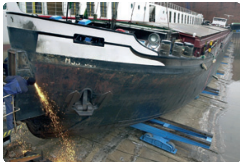
This inclined slide track, on which the heavy ship will glide into the water when it is launched, is painted with a special soap to reduce friction.
